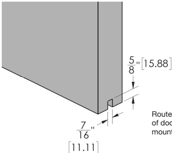
Route bottom, full length of door to receive floor mounted guide.
