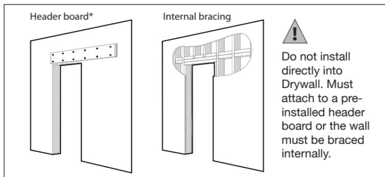
\*Header board and anchor screws not included.
