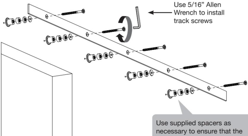
Use 5/16" Allen Wrench to install track screws
