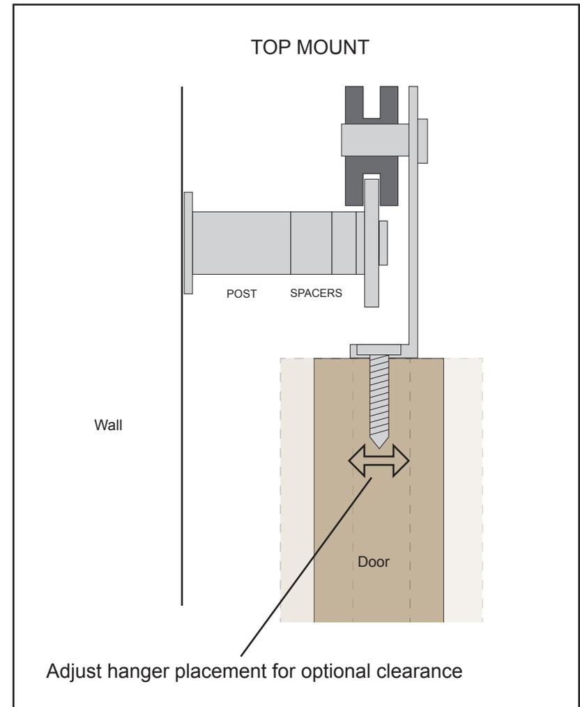
The wall or structure that your system will be mounted on must be designed to support a maximum door weight of 400 lbs.
