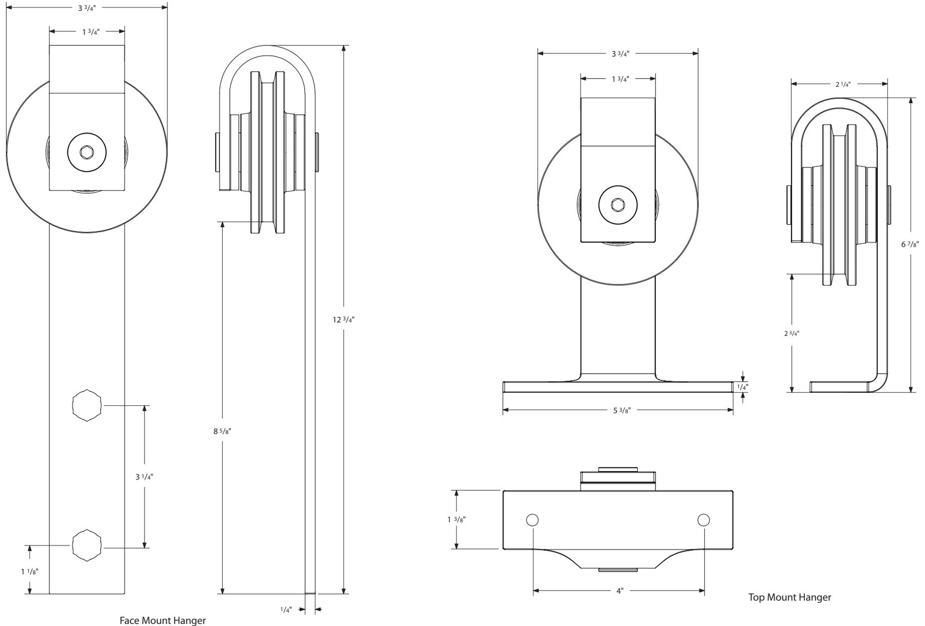
The wall or structure that your system will be mounted on must be designed to support a maximum door weight of 400 lbs.
