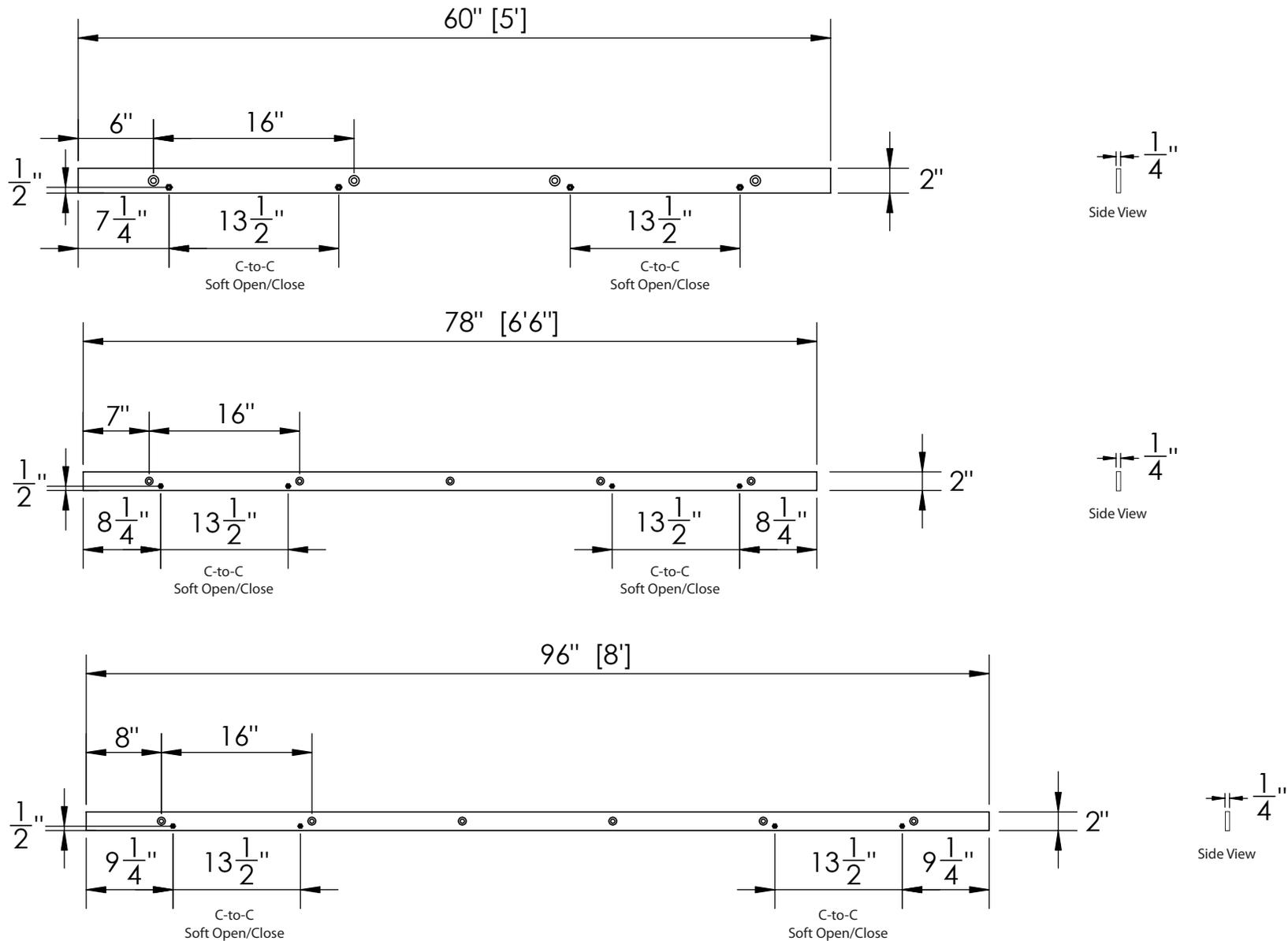
The wall or structure that your system will be mounted on must be designed to support a maximum door weight of 400 lbs.
