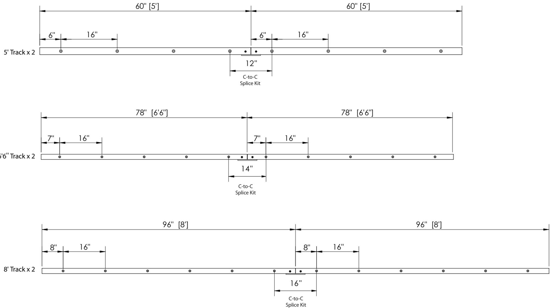
The wall or structure that your system will be mounted on must be designed to support a maximum door weight of 400 lbs.
