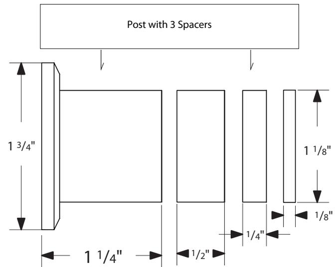
Without a counterbore, the door thickness is 1-3/8" to 2-1/4"
