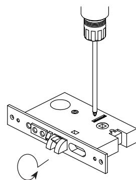
2. Pull out and rotate latch bolt to reverse its direction.
