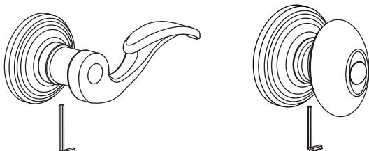
Tighten Set screw at bottom of lever or knob.
