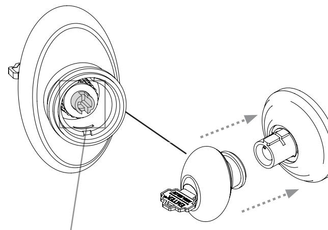
Before inserting knob/lever onto stem, make sure cylinder tailpiece is vertical as shown.
